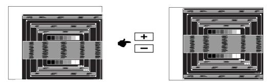
6 1) Adjust the H.Position so that the left side of the picture frame will move to the left edge of the display area.
