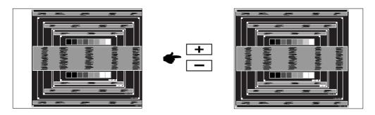
2) Stretch the right side of the picture frame to the right edge of the display area by adjusting the Pixel Clock.
