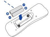
3 Replace the battery cover in the direction of the arrow and snap it back into place.
